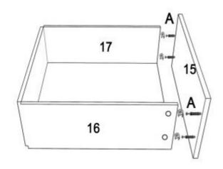
USE HARDWARE A (X4 SETS) TO CONNECT DRAWER FRONT PANEL (15)TO THE DRAWER FRAME INSTALLED IN STEP 2.
