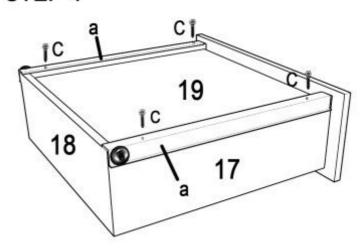
USE THE SCREW C (X4PCS) TO ATTACH THE a PART OF THE HARDWARE B TO THE SIDES OF THE DRAWER..
