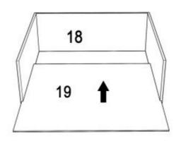
LOAD DRAWER BOTTOM PLATE(19) INTO THE DRAWER FRAME INSTALLED IN STEP 1.
