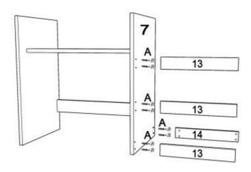
AS SHOWN IN THE FIGURE, USE HARDWARE A(X8SETS) TO CONNECT ONE END OF THE HORIZONTAL PLATES 13 AND 14 TO THE SIDE PLATE 7.
