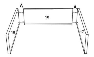
USE HARDWARE A (X4 SETS)TO CONNECT DRAWER LEFT PANEL (16), DRAWER RIGHT PANEL (17) AND DRAWER REAR PANEL(18) RESPECTIVELY.
