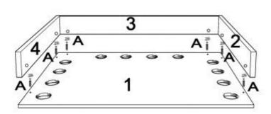
AS SHOWN IN THE FIGURE, INSTALL THE MIRROR(1) ON THE FRAME ASSEMBLED IN STEP 12 AND CONNECT IT WITH HARDWARE A.
