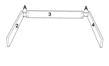
AS SHOWN IN THE FIGURE, USE HARDWARE A (X4SETS)TO CONNECT THE TWO ENDS OF THE MIRROR UPPER FRAME (3) WITH THE MIRROR SIDE PLATES 2, 4 RESPECTIVELY.
