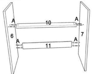
AS SHOWN IN THE FIGURE, USE HARDWARE A(X8SETS) TO CONNECT THE TWO ENDS OF THE HORIZONTAL PLATES 10 AND 11 TO THE SIDE PLATES 6 AND 7 RESPECTIVELY
