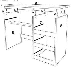
AS SHOWN IN THE FIGURE, INSTALL THE HARDWARE A(X5SETS) TO THE SIDE AS SHOWN IN THE FIGURE, INSTALL THE DESKTOP ASSEMBLED IN STEP 9 TO PANELS 9, 12 ON THE DESKTOP BOARD (5).
