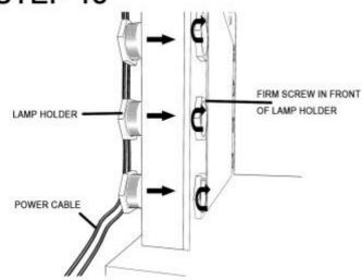
AS SHOWN IN THE FIGURE, TAKE OUT THE LAMP ASSEMBLY AND REMOVE THE BULB, THEN REMOVE THE FRONT SOLID SCREWS OF THE LAMP HOLDER, AND THEN INSTALL THE LAMP HOLDERS INTO THE HOLES UNDER THE MIRROR ONE BY ONE, AND INSTALL THE FRONT SOLID SCREWS ON THE LAMP HOLDER.
