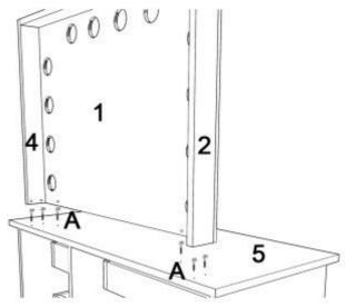
AS SHOWN IN THE FIGURE, INSTALL THE MIRROR ASSEMBLED IN STEP 13 ON THE TOP OF THE DRESSING TABLE ASSEMBLED IN STEP 11 AND CONNECT IT WITH HARDWARE A(X6SETS).
