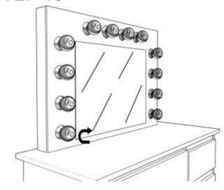
AS SHOWN IN THE FIGURE, INSTALL ALL THE BULBS INTO THE SOCKET IN A CLOCKWISE DIRECTION,
